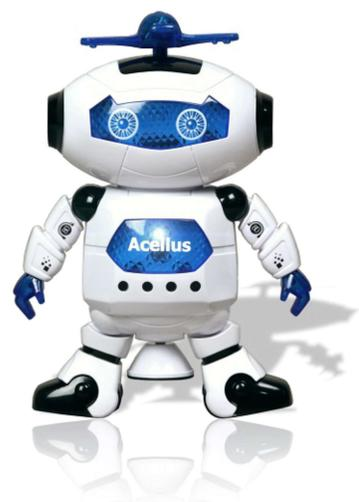
*Figure 13: Cellus Bot is a teaching robot equipped with lights, motor, and sensors, all controlled by block coding modules included in the course. Students first learn how to control the robot in the most simplistic manner, but the lessons develop in complexity as the course progresses.*
